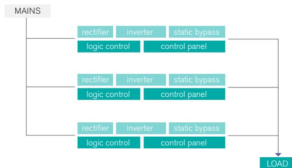
Newave's modular DPA UPScale ST is built of self-contained modules that include the entire UPS hardware and software; hence, it eliminates all the common parts which are potential single points of failure.
